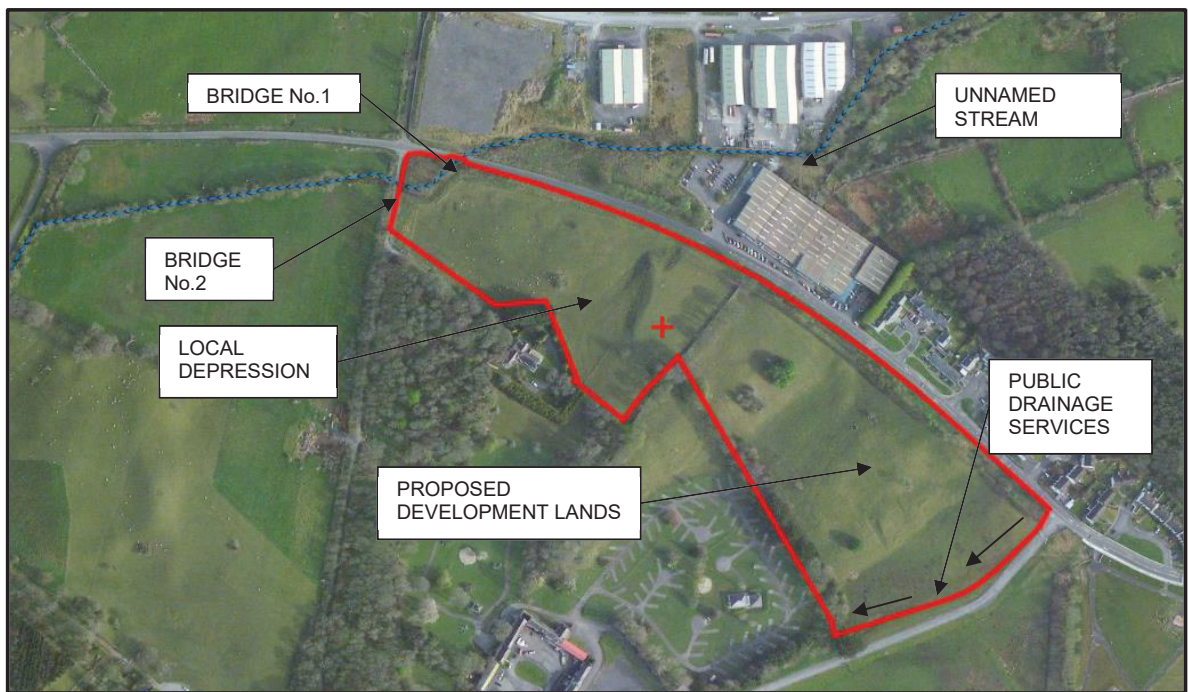
Figure 2.3 Local drainage network overview
