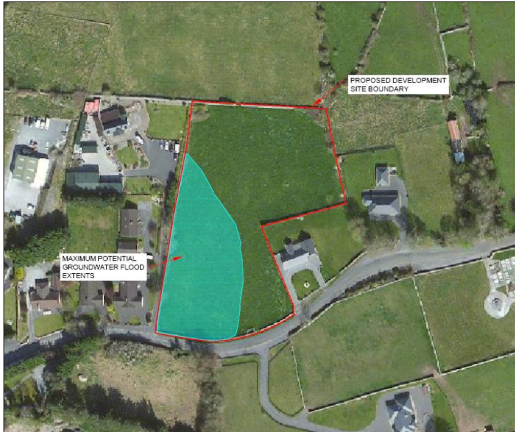
Plate 2-1 - Floodable area within the southwest of the site (blue, Flood Zone A). Source: Priority Geotechnical Ltd. - Flood Risk Assessment Report.
