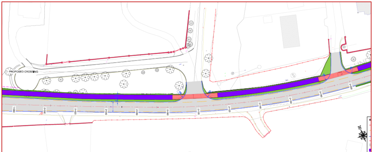
Figure 6.2: Typical Layout of Two-Way Shared Facility Crossing at Junctions and Direct Accesses
