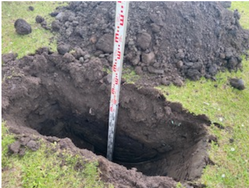
Trial Hole No 3 – Clay/Waste material mix to 750mm below surface
