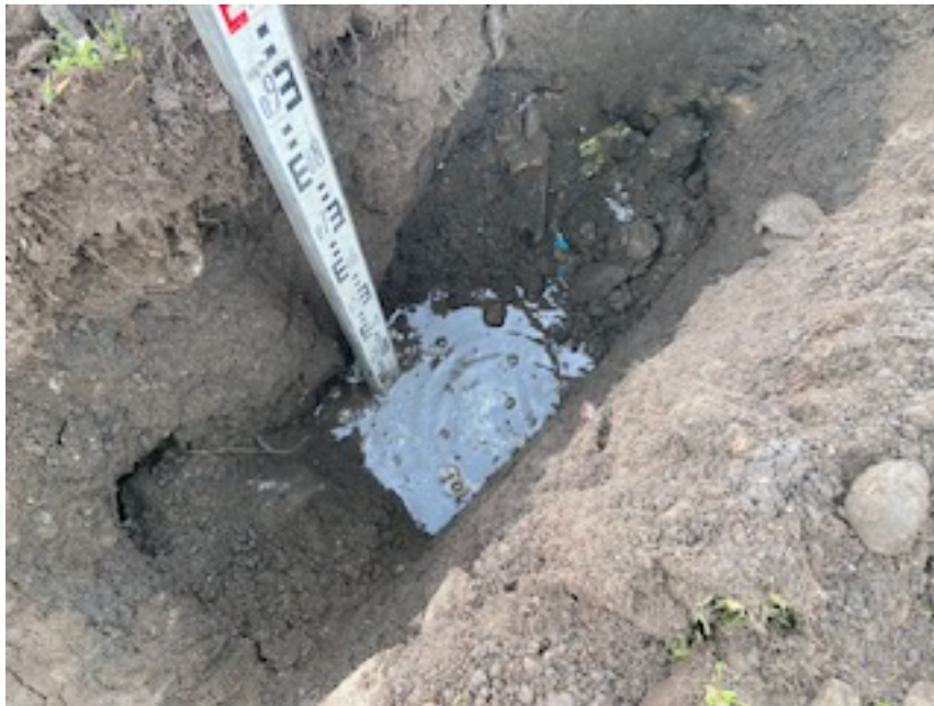
Trial Hole No 6 – Water table at 800mm below surface
