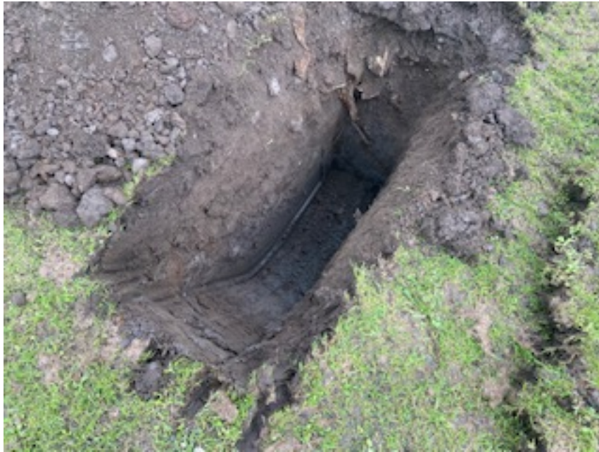
Trial Hole No 1 – Clay/Waste material mix to 850mm below surface
