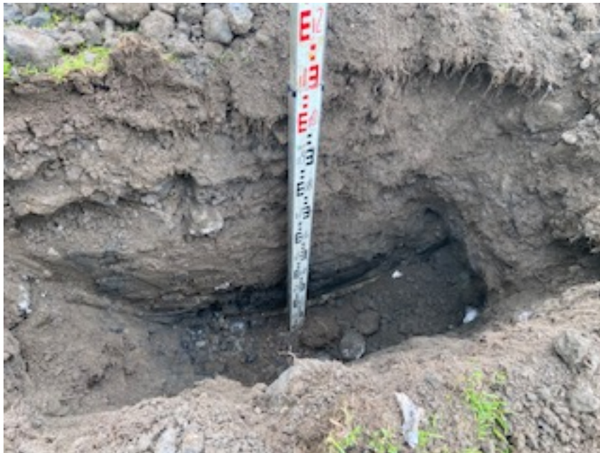
Trial Hole No 4 – Clay/Waste material mix to 700mm below surface
