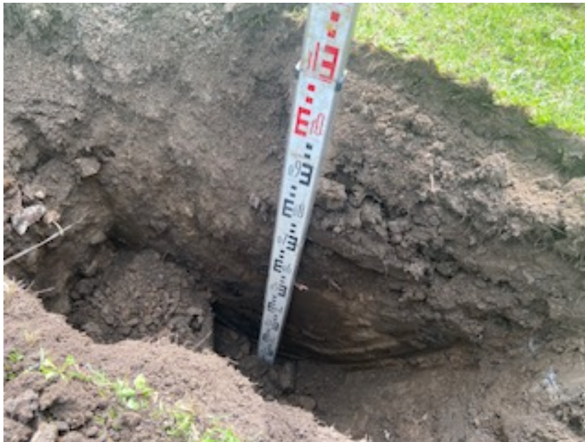
Trial Hole No 2 – Clay/Waste material mix to 750mm below surface
