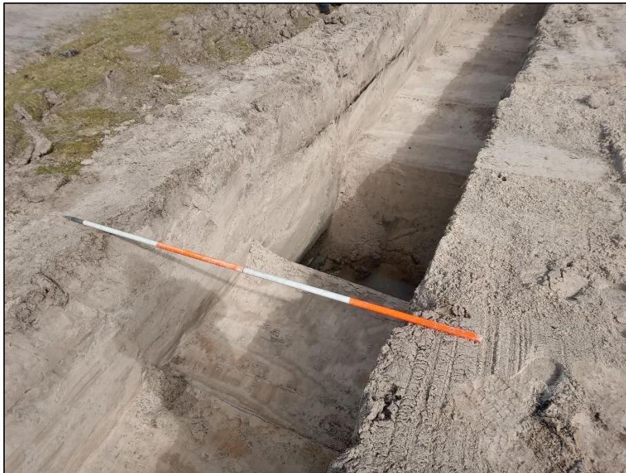
Plate 4 Water seeping into base of Test Trench 5 with water table reached at 3m
