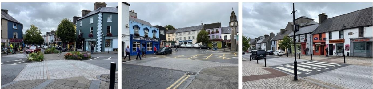
Figure 7-8 – Examples of raised uncontrolled crossings and James Street zebra crossing in the town centre
