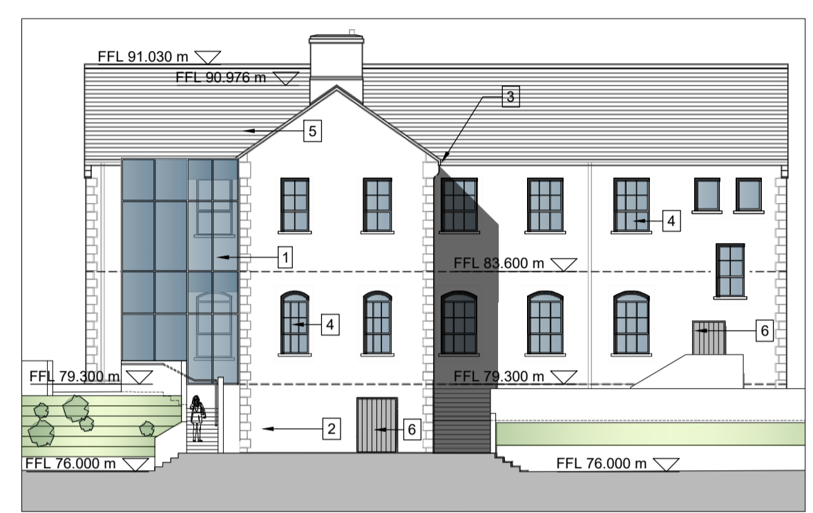
PROPOSED NORTH -WEST ELEVATION SCALE 1:200
