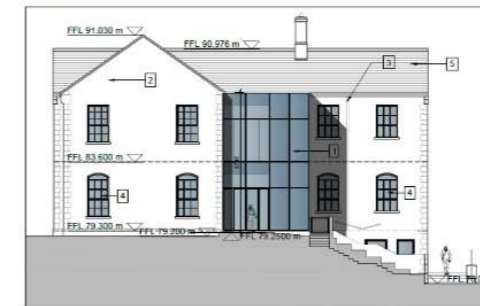
PROPOSED NORTH-EAST ELEVATION SCALE 1:200
