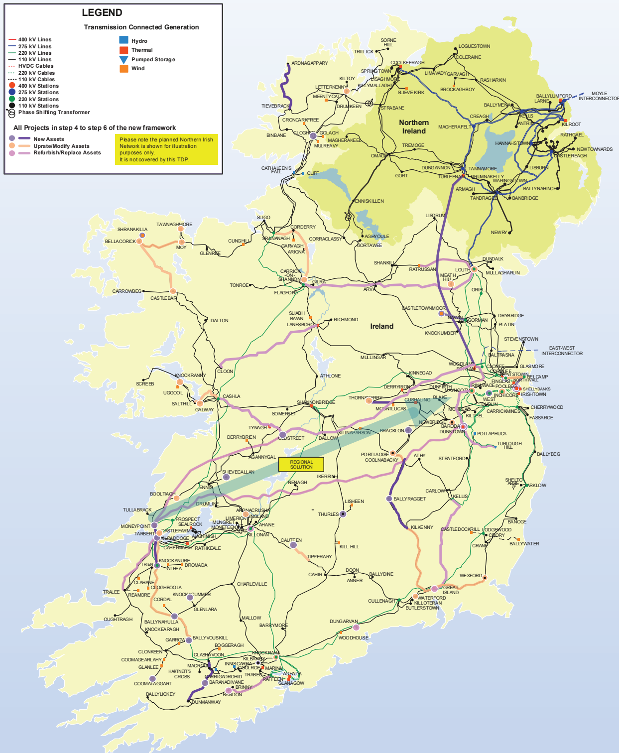
Figure 64: Electrical Transmission System
