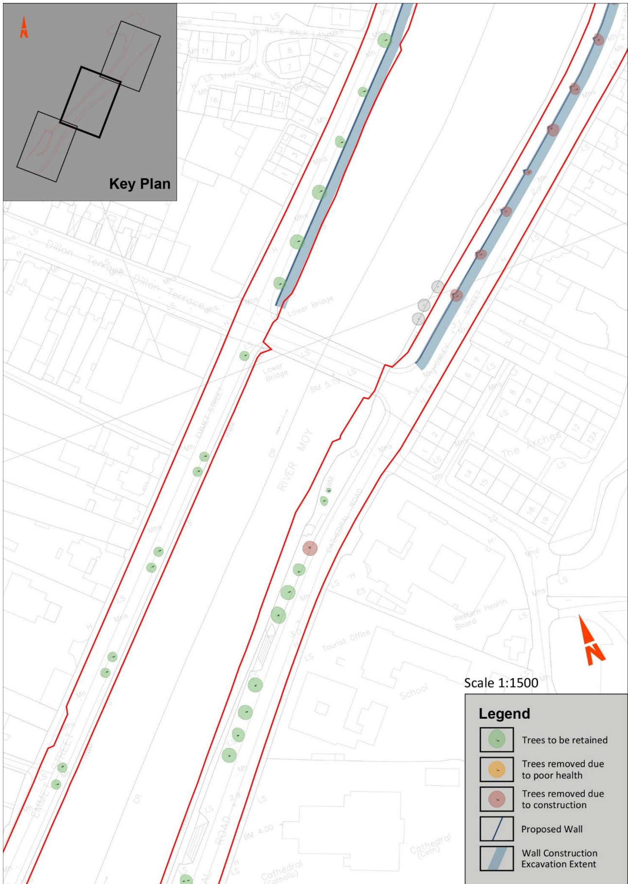
Figure 19-8: Proposed Construction and Impacts on Existing Trees Along the River Moy (Central Section)
